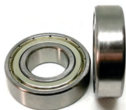
LS/C-1026 BALERO 6004ZZ, CENTRO 20MM, DIAMETRO 42MM, ALTURA 12MM
