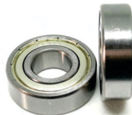
LS/C-1030 BALERO 6203ZZ, CENTRO 17MM, DIAMETRO 40MM, ALTURA 12MM
