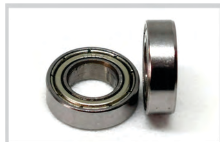
LS/C-1019 BALERO 689Z, CENTRO 9MM, DIAMETRO 17MM, ALTURA 5MM
