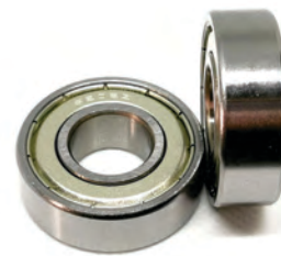
LS/C-1025 BALERO 6202ZZ, CENTRO 15MM, DIAMETRO 35MM, ALTURA 11MM
