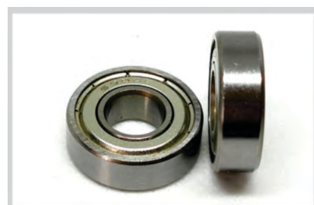
LS/C-1014 BALERO 698Z, CENTRO 8MM, DIAMETRO 19MM, ALTURA 6MM
